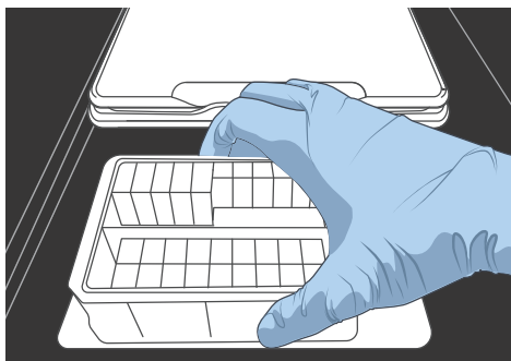
Figure 8 Placing DNB Load Plate
