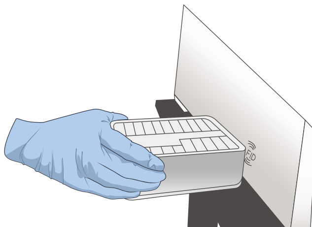
Figure 7 RFID scanning area of DNB Load Plate
